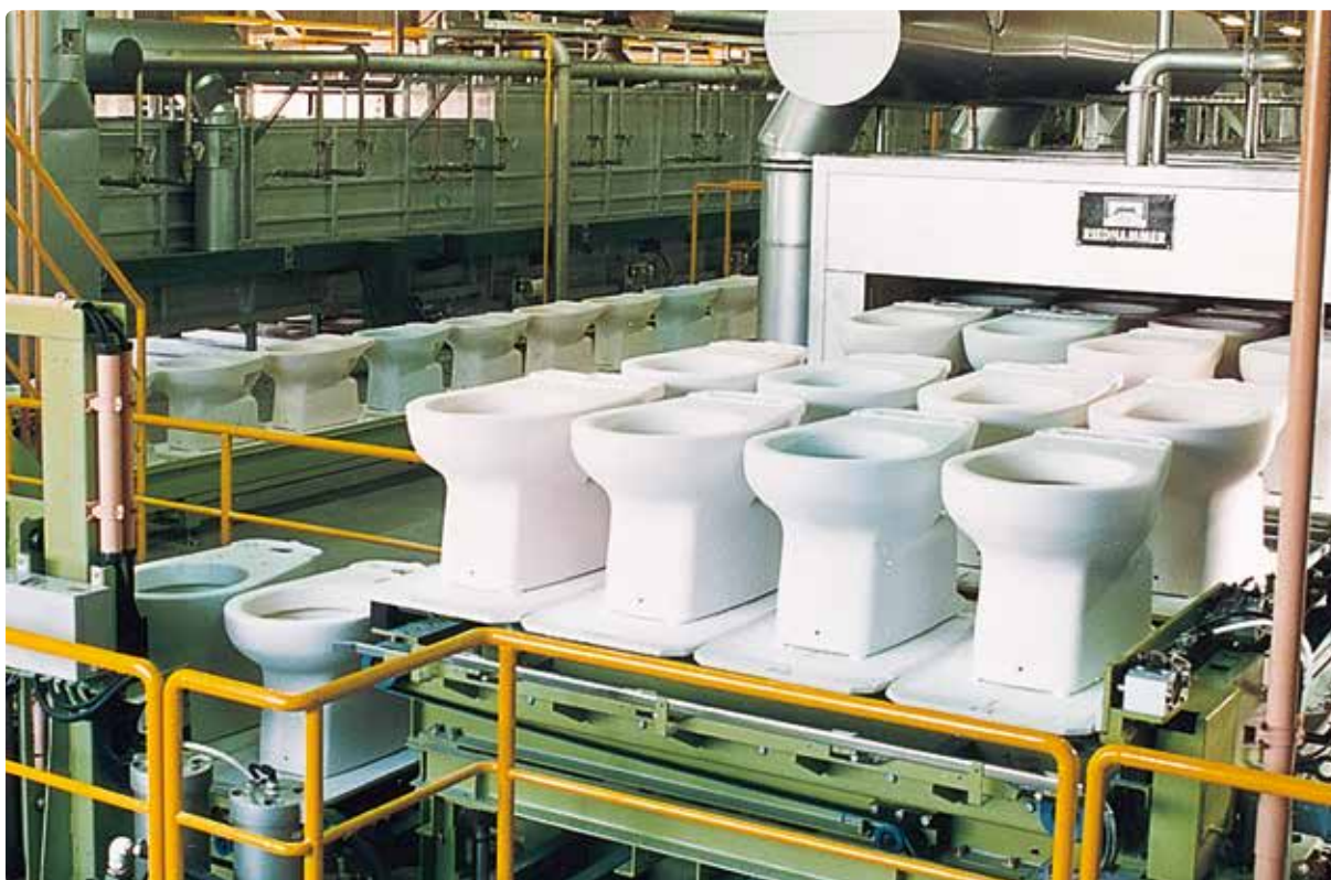
Entrance of TRS – gas-heated for sanitary ware first firing
