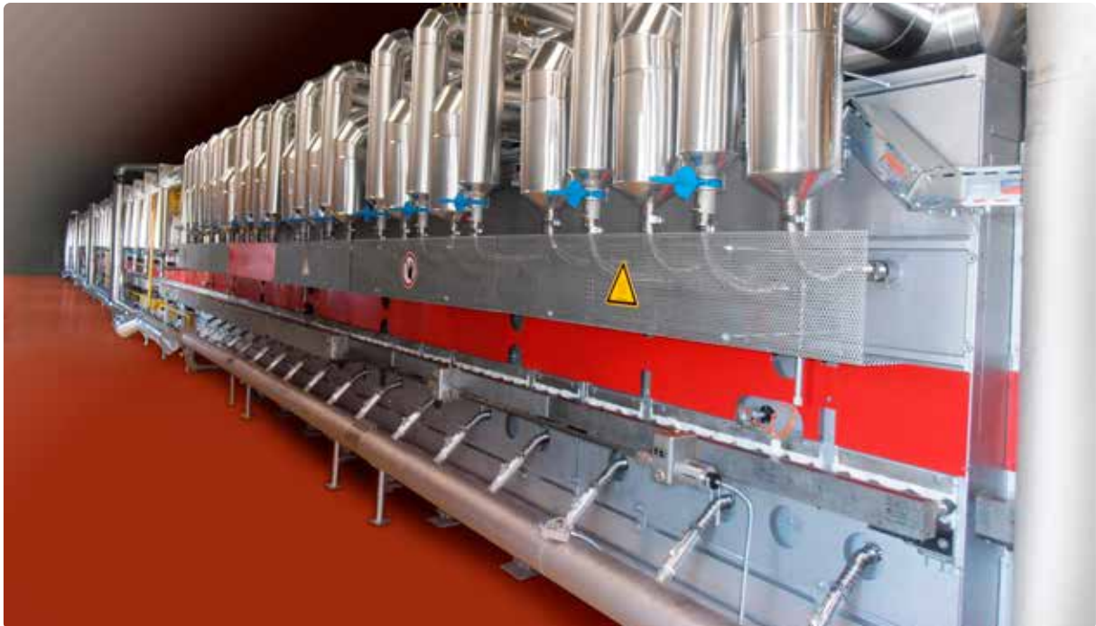
ROLLER KILN Roller kiln for first firing and re-firing of Sanitaryware
