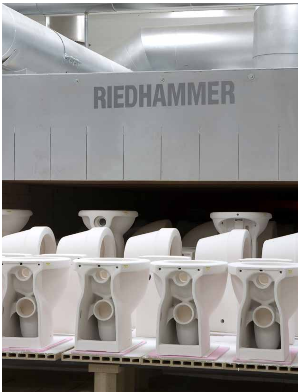
TUNNEL KILN Tunnel kiln for first firing and re-firing of Sanitaryware
