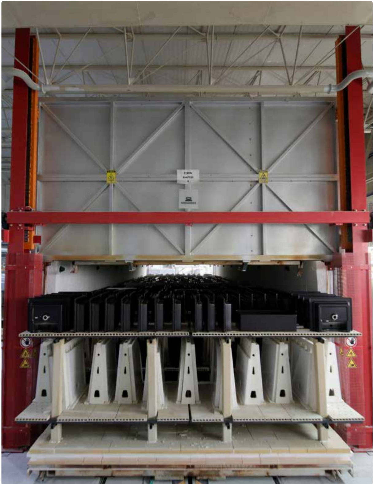
SHUTTLE KILN Shuttle kiln for first firing and re-firing of Sanitaryware
