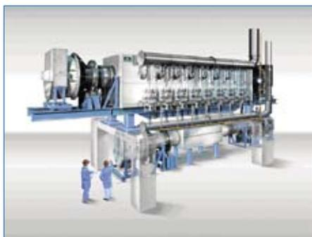
Fig. 3 • Indirectly heated rotary kiln with atmosphere control
