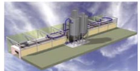
This Galician producer of hollow bricks will count in the next weeks with a solid fuel firing system model MICROMATIC that will use petroleum coke as the main fuel in the kiln, for an output of approx. 250 tm/d. The fuel used in the preheating zone will be natural gas.
