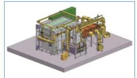
Fig. 7 • Shuttle kiln plant with low O<sub>2</sub> technology
