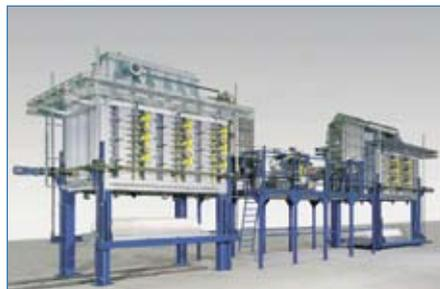
Fig. 4 • Two electrically heated gas-tight top-hat kilns
