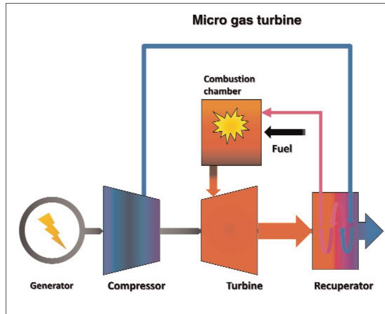
**Fig. 3** Functional diagram of the micro-gas turbine
