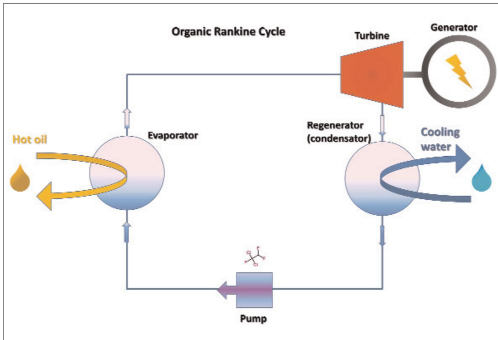
Fig. 1 Functional diagram of the ORC process
