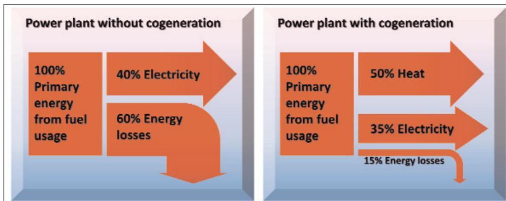
Fig. 2 Power plant without cogeneration vs. power plant with cogeneration
