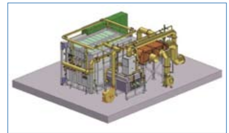
Fig. 7 • Shuttle kiln plant with low O 2 technology
